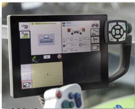
ISOBUS tractor monitor example
